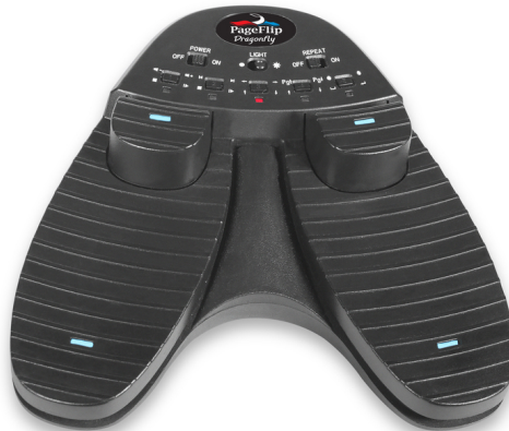
Figure 8: Primary (larger) and secondary (smaller) pedals. Each of these four pedals has an LED light that can be turned on for use in dim venues.
